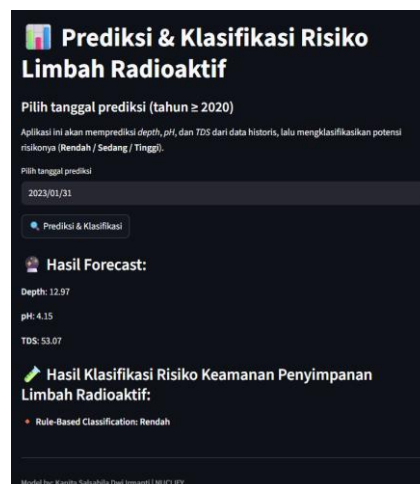
Figure 8. Result of Forecasting Time-Series and Rule-Based Classification
