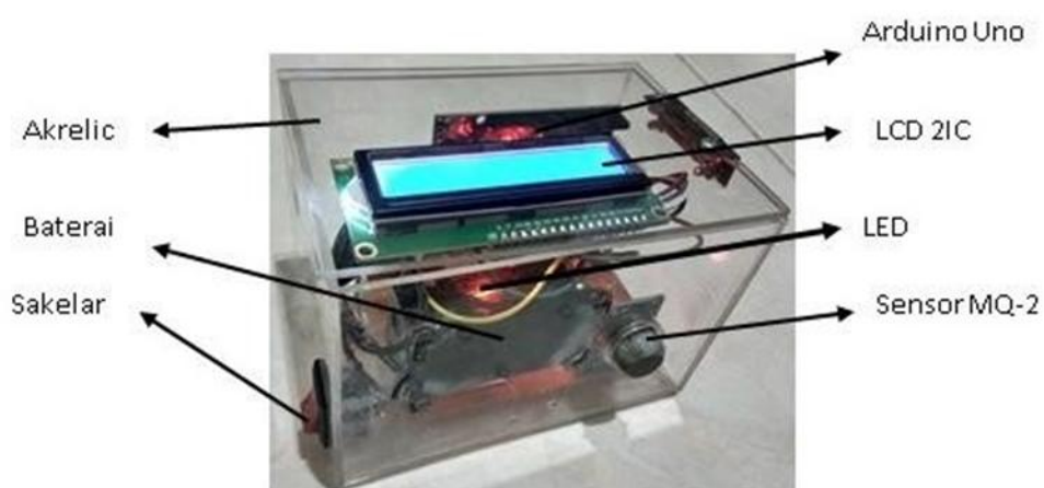
Gambar I. 1 Alat peraga pendeteksi kebocoran Gas (LPG) Otomatis Berbasis Arduino
