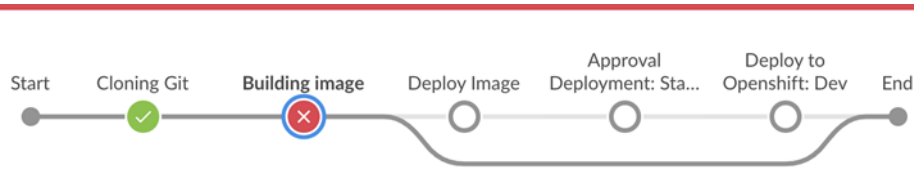
Gambar 3.4. Proses Pipeline Gagal pada stage Building Image
