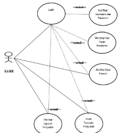
Gambar 2. Use Case Diagram Halaman Kasir
