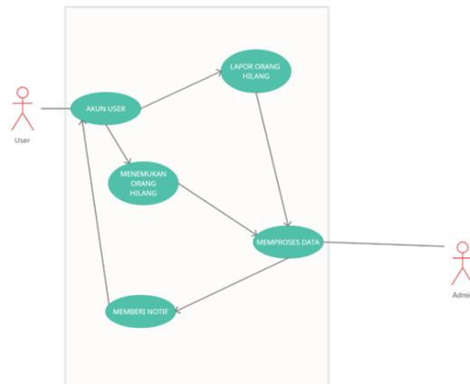
**Gambar 4.** Use Case Diagram Portalang
