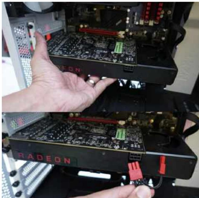
Gambar 54. Memasang VGA card
