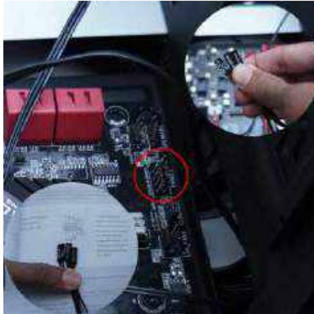
Gambar 51. Memasang Front panel
