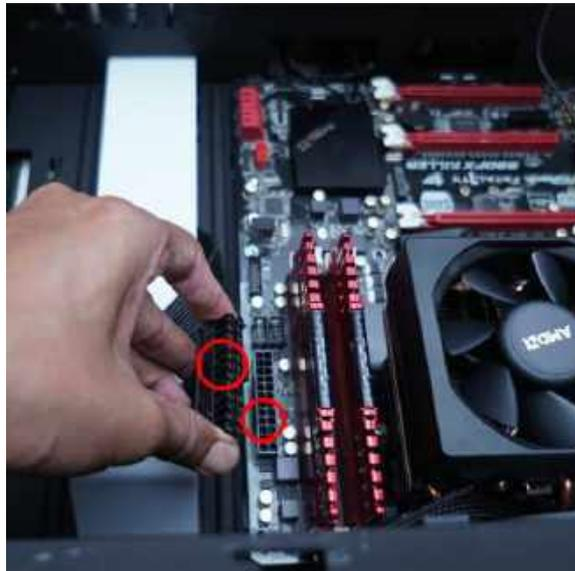
Gambar 49. Memasang kabel motherboard 24 pin
